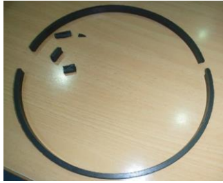
Gambar 22. Kerusakan Seal As (8C-9182)
