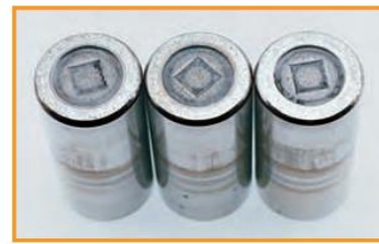
Roller end scoring — Metal-to-metal contact from breakdown of lubricant film. Gambar 10 scoring pada roller Courtesy The Timken Co.
