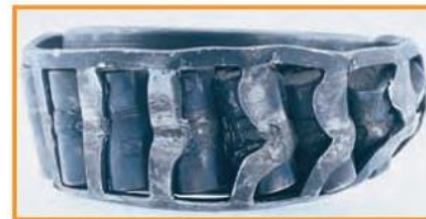
Total bearing lock-up — Rollers skew, slide sideways and lock-up bearing. Gambar 12 bearing macet Courtesy The Timken Co.
