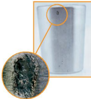
Gambar 9 electric arc pitting Courtesy The Timken Co.
