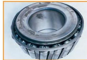
Cone large rib face deformation — Metal flow from excessive heat generation. Gambar 11 sangkar terdeformasi Courtesy The Timken Co.
