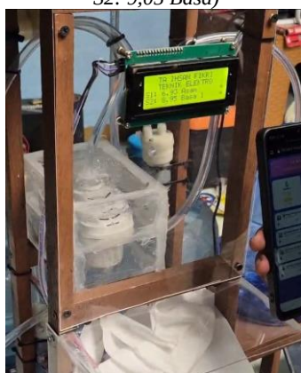
Gambar 4.5 Tampilan LCD percobaan 2 (S1: 6,93 Asam; S2: 8,95 Basa)
