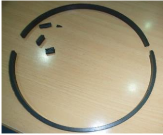
Gambar 22. Kerusakan Seal As (8C-9182)
