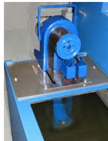
Gambar 2.1. (a) Disk skimmer dan (b) Belt skimmer
