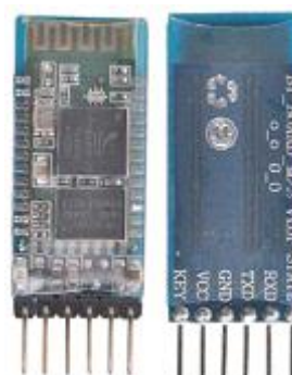
Gambar 3. Modul Bluetooth HC-05
