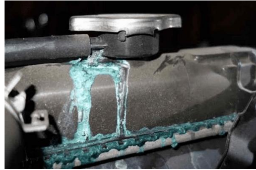
Gambar 6. Selang Input Radiator Bocor
