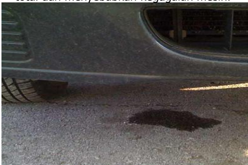
Gambar 12. Tanda Kebocoran Radiator
