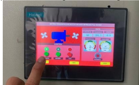
Gambar 15. Pengujian Kontrol Forward HMI
