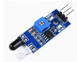
Gbr. 2 Sensor Infrared (IR)
